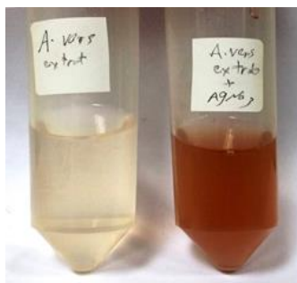
Fig. 1 – Color of A. versicolor free cell extract without AgNO 3 (A) and with AgNO 3 (B)
